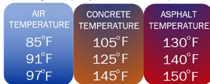
Figure 5. Impact of Heat on Concrete and Asphalt
